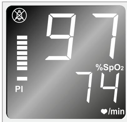
The frequency of the pulse tone is closely related with saturation level; lower tones indicate lower saturation levels.
