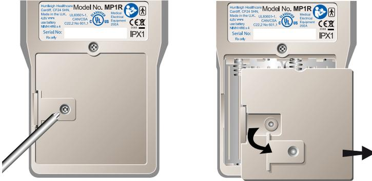
1. Remove the securing screw and the battery cover.
