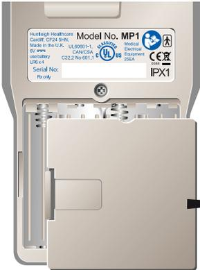
1. Slide the battery compartment latch across to remove the battery cover.
